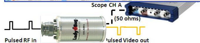
Measuring Opt 0W2 Wideband, Negative Detector, Analog Video Output Signal
