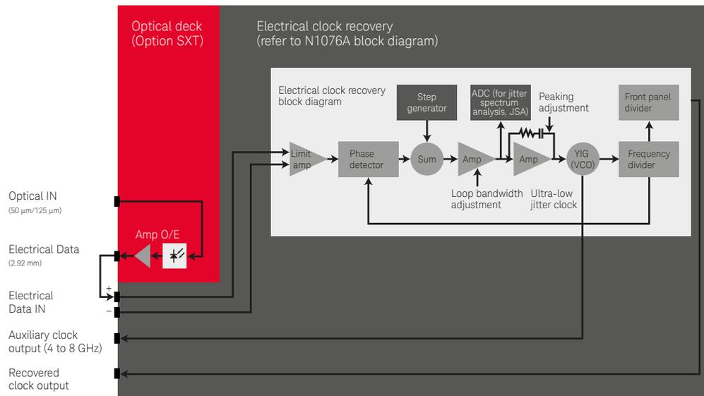
Figure 9. The N1077A with Option SXT combines an integrated amplified O/E with an instrument-grade electrical clock recovery circuit (user supplies an external optical splitter as necessary).
