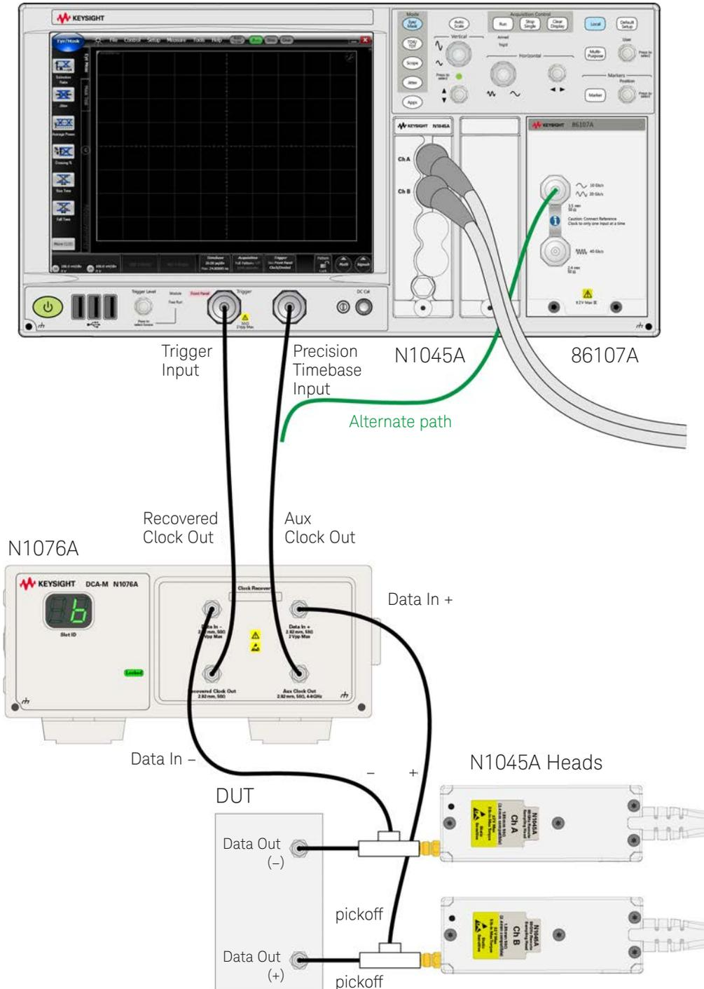
Figure 14. Connection diagram showing an N1076A connected to an 86100D DCA-X and remote head modules using high-bandwidth electrical pick-offs (optional accessory).
