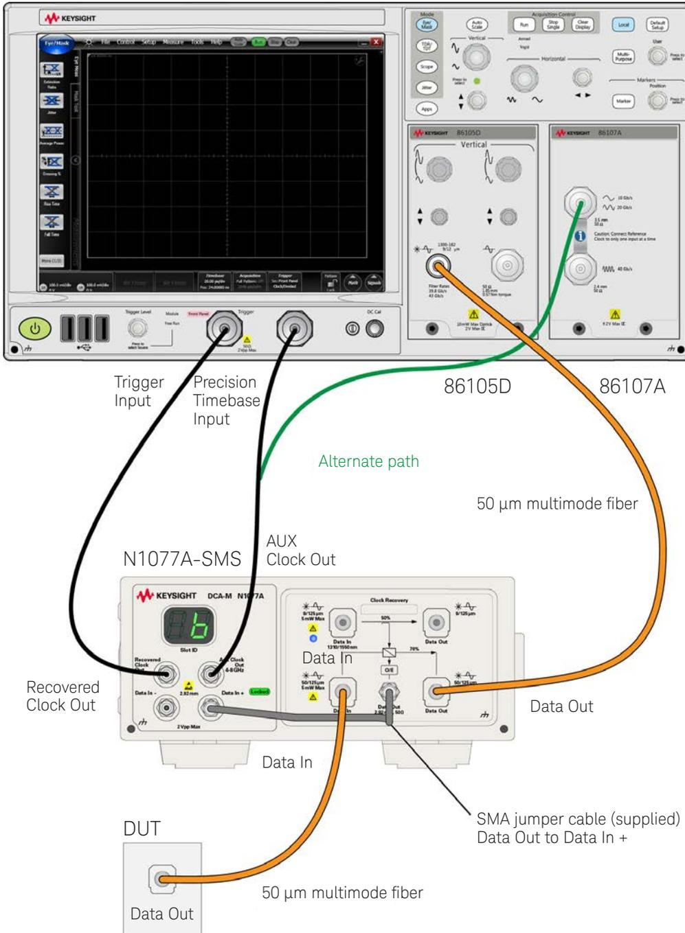
Figure 16. Connection diagram showing an N1077A with Option SMS connected to an 86100D DCA-X mainframe (precision timebase is optional) and 86105C/D wide-wavelength plug-in module.
