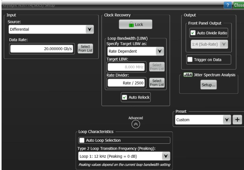
Figure 12. Easily configure the N1076A/77A clock recovery data rate, loop bandwidth, and peaking using the N1010A FlexDCA user interface running on an 86100D DCA-X mainframe or standalone PC.
