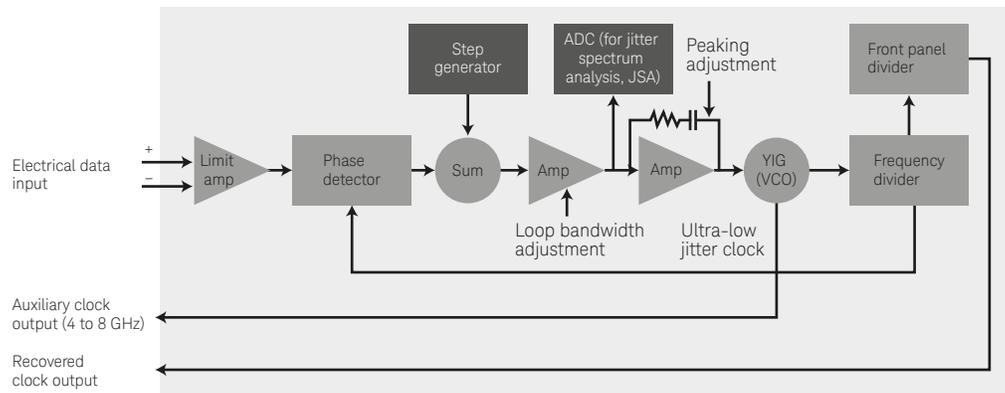
Figure 5. As shown in this block diagram of the electrical clock recovery, the N1076A recovers clock signals from NRZ and PAM4 input signals, and provides jitter analysis capability (Option JSA) for additional insight and measurement accuracy.
