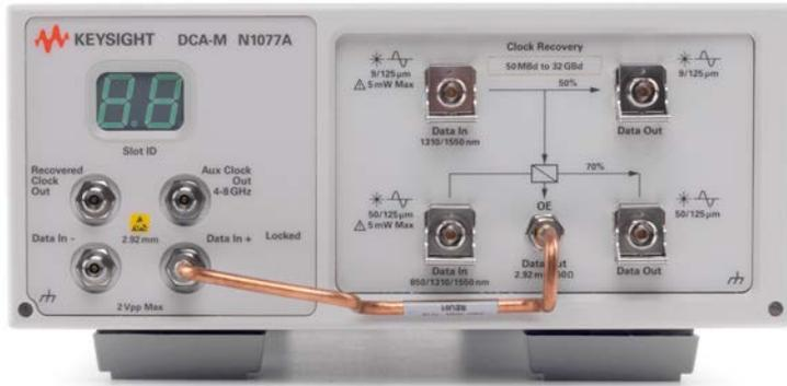
Figure 6. The N1077A recovers clock from both electrical and 850 to 1550 nm optical signals operating from 50 MBaud to 32 GBaud.
