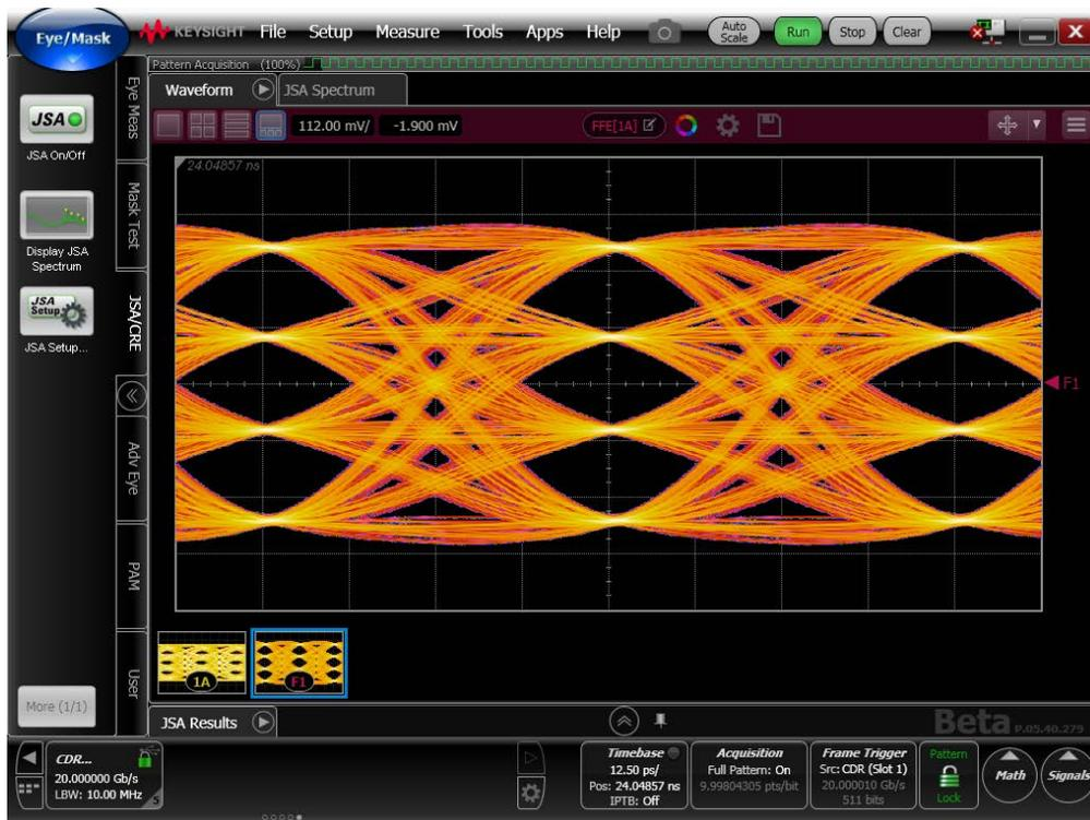
Figure 10. The N1076A/77A provides clock recovery capabilities for NRZ (top) and PAM4 (bottom) signals.
