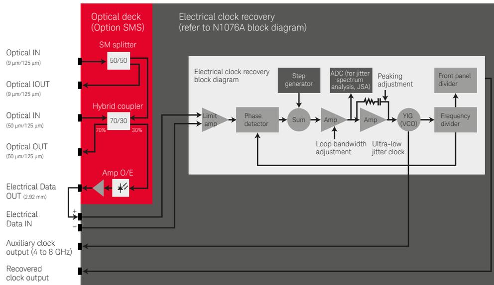
Figure 7. The N1077A with Option SMS combines an integrated optical deck (a splitter, bulk-optics coupler, and an amplified O/E) with an instrument-grade electrical clock recovery circuit.
