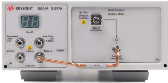
Figure 8. The N1077A with Option SXT recovers a clock from both electrical and optical (850 to 1550 nm) signals operating from 50 MBaud to 32 GBaud. Instead of an integrated optical splitter, Option SXT units allow users to provide their own external optical splitters having a split ratio optimized for their particular setup.
