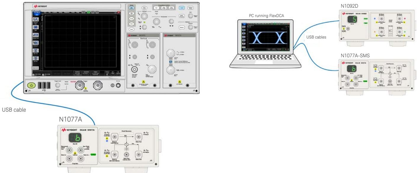
Figure 13. The N1076A/77A clock recovery instrument is controlled via a rear-panel USB connection to an 86100D DCA-X mainframe (left), or to a standalone PC (right) running the N1010A FlexDCA user interface.
