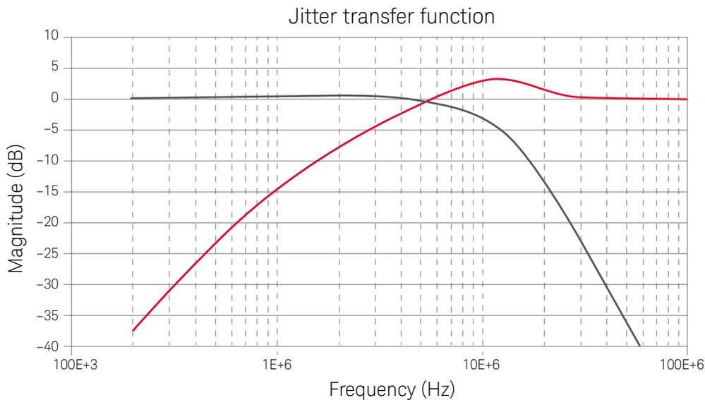
Figure 1. The N1076A/77A clock recovery may be configured as a jitter receiver when characterizing phase-locked loop (PLL) designs using 86100DU-400 PLL analysis software.
