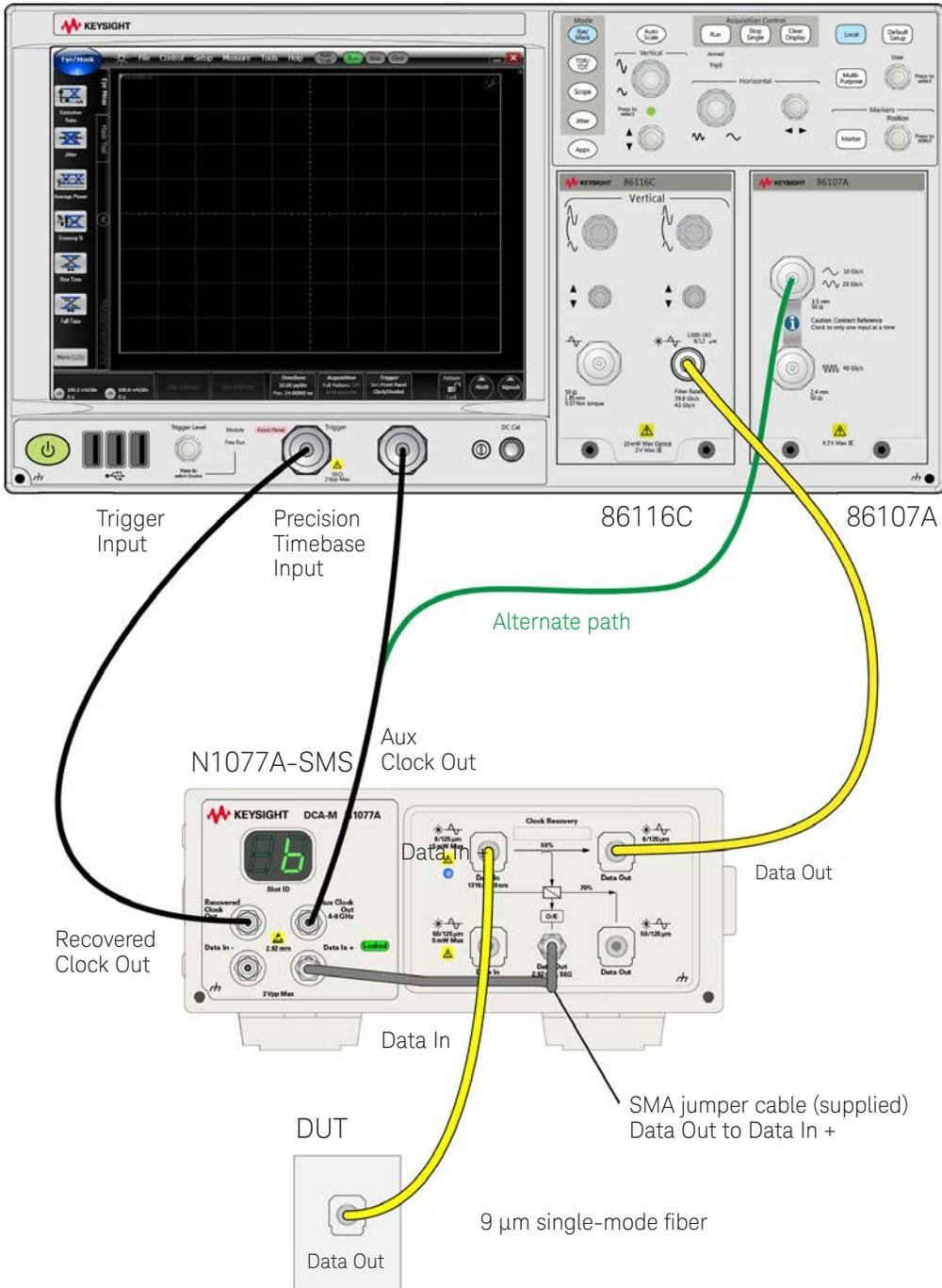
Figure 17. Connection diagram showing an N1077A with Option SMS connected to an 86100D DCA-X mainframe (precision timebase is optional) and 86116C single-mode plug-in module.
